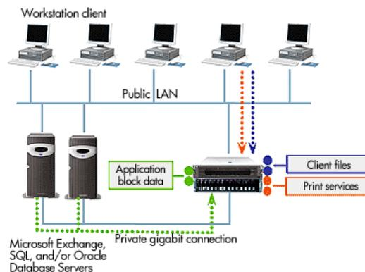
Figure 4: Network Attached Storage<sup>27</sup>
